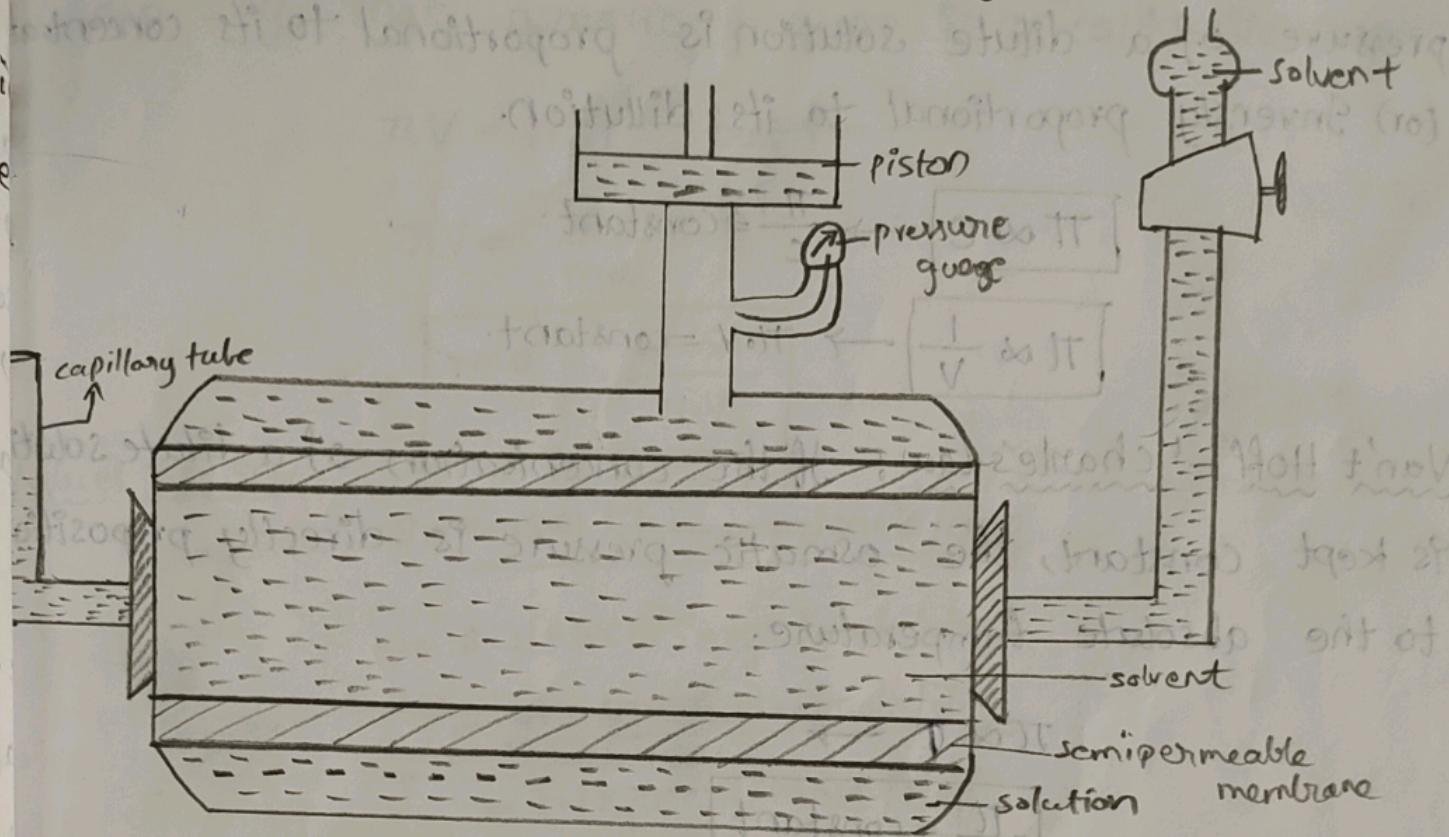
This method involves the determination of the excess pressure that is applied upon the solvent to prevent the entry of the solvent in to the solution.
