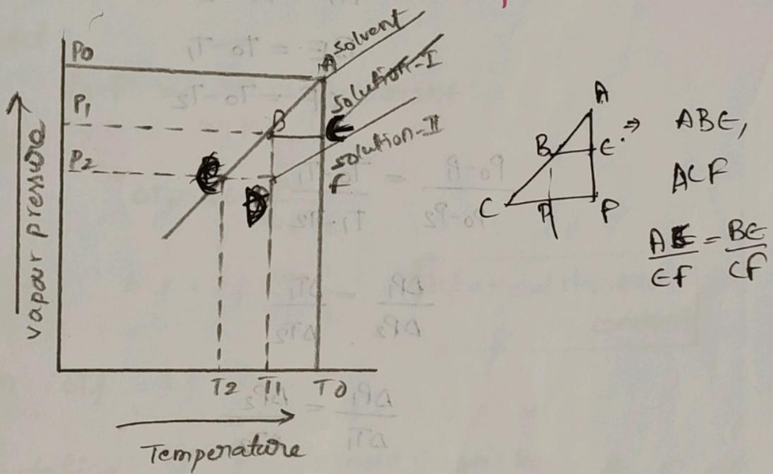
Study the freezing point curves, consider solvent. solution-I & solution-II. The vapour pressure and temperature curves of this systems are as shown in the graph. from the graph point A represents the equilibrium b/w solid and liquid of pure solvent similarly the points B & C represents the freezing points of solution-I & solution-II. Let us consider  $P_0, P_1, P_2$  are the vapour pressures of pure solvent, solution-I & solution-II.
