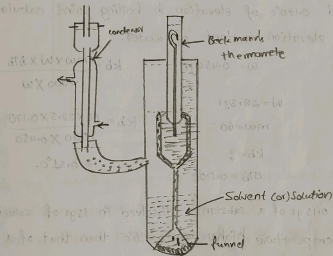
Cottrell's apparatus consists of graduated boiling tube containing solvent or solution, a condenser fitted. In the slide tube of the main graduated tube, the condenser returns the vapourised solvent to the boiling tube.
