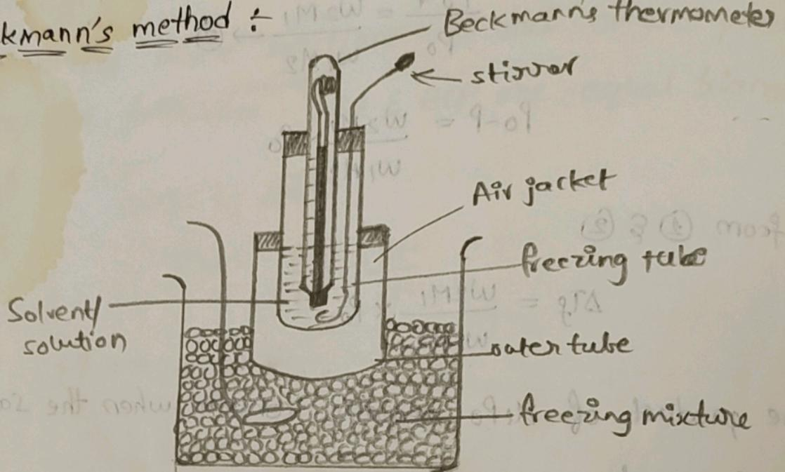
The inner freezing tube fitted with a beckmann thermometer and a platinum stirrer. The outer glass tube is fitted the inner freezing tube, leaving an air space between them. A glass jar containing a suitable freezing mixture whose F.P is about  $5^{\circ}\text{C}$  lower than that of the pure solvent.
