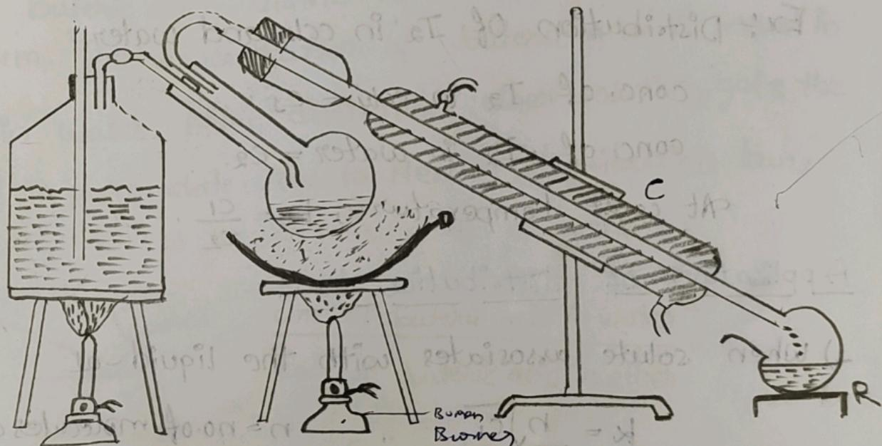
As in the above distillation diagram the flask containing impure liquid to be purified is slowly heated and a current of steam picks up the volatile substance from the liquid and passes it in to the condenser. The steam liquid vapours condense in the condenser and thus trickle down in the receiver.
